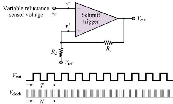
**Figure 16.25** Signal processing for a 60-tooth-wheel RPM sensor
