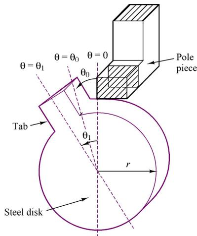
**Figure 16.26** Reluctance sensor for measurement of angular position
