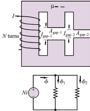
**Figure 16.22** Magnetic structure with two air gaps
