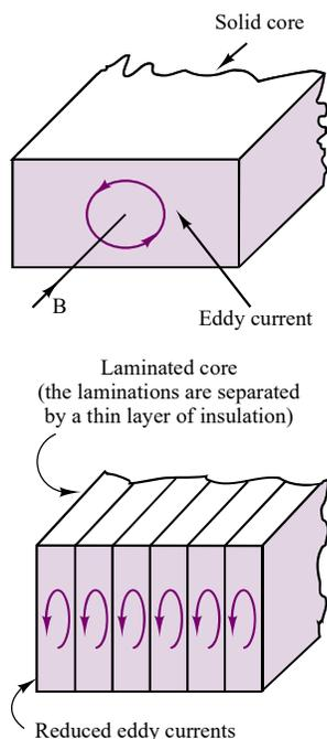
**Figure 16.31** Eddy currents in magnetic structures
