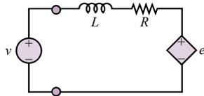
**Figure 16.55** Model of transducer electrical side
