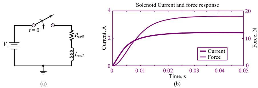
**Figure 16.42** Solenoid equivalent electrical circuit and step response
