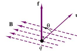
**Figure 16.2** Charge moving in a constant magnetic field
