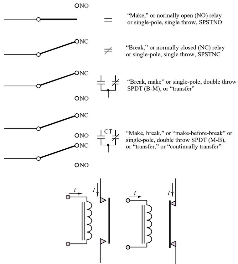
Basic operation of the electromechanical relay: The (small) coil current  $i$  causes the relay to close (or open) and enables (interrupts) the larger current,  $I$ .
