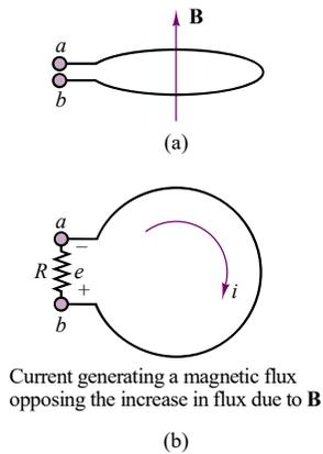
Figure 16.4 Flux direction
