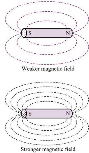
**Figure 16.1** Lines of force in a magnetic field
