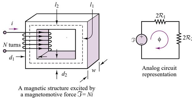
**Figure 16.13** Analogy between magnetic and electric circuits
