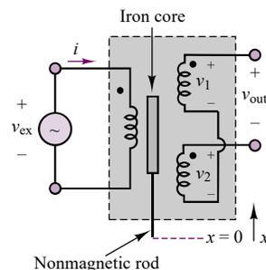
**Figure 16.7** Linear variable differential transformer
