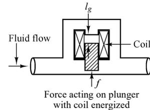
**Figure 16.39** Application of the solenoid as a valve
