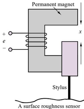
**Figure P16.36** A surface roughness sensor
