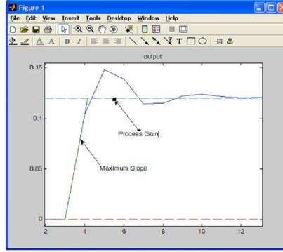
Figure 8. Reaction curve technique
