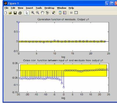
Figure 7. Cross correlation function between input  $u_1$  and output  $y_1$
