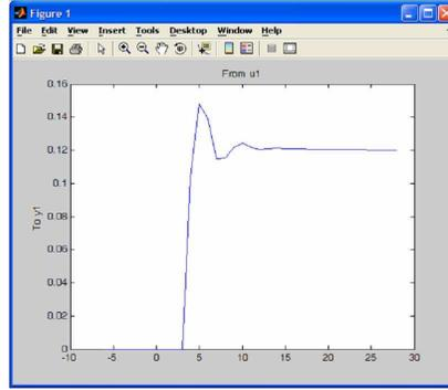
Figure 10. Step response of the identified model
