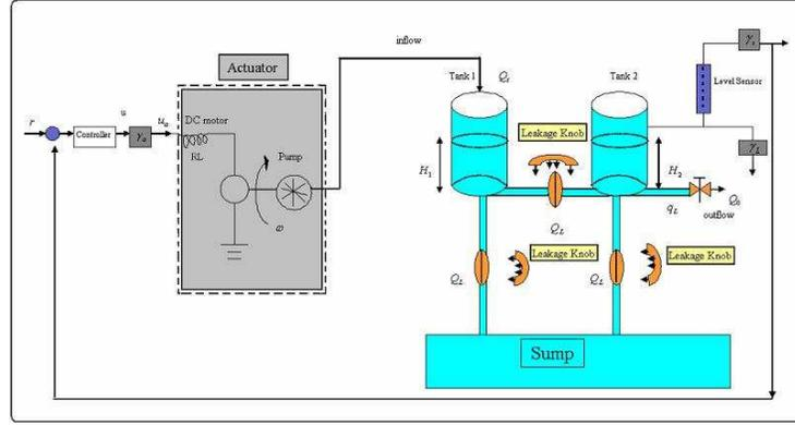
Figure 2. Two-tank fluid control system
