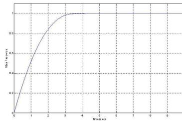
Figure 20. Step response with second order sliding mode control
