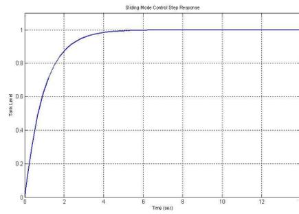
Figure 19. Step response of the identified model using sliding mode control
