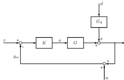
Figure 16. Closed loop system
