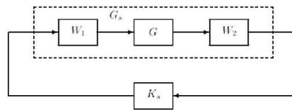
Figure 14. Loop shaping design procedure implementation
