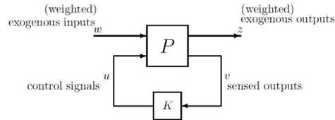
Figure 13. General control configuration for  $\mathcal{H}_\infty$  control
