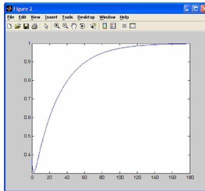
Figure 12. Closed loop response for PID controller
