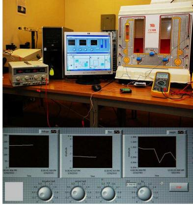
Figure 3. Top Figure: The two tank system interfaced with the Labview through a DAQ and the amplifier for the magnified voltage, Bottom Figure: The labview setup of the apparatus including the circuit window and the block diagram of the experiment.
