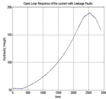
Figure 11. Open loop response of the system with leakage faults
