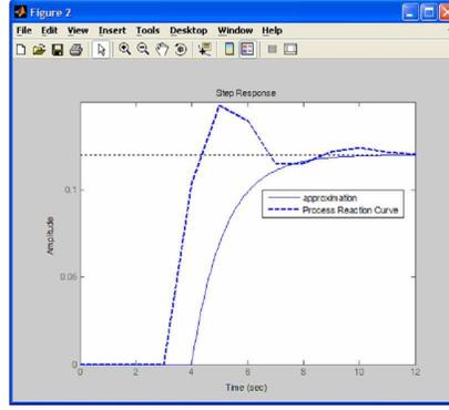
Figure 9. Comparison of model approximation and the original step response model
