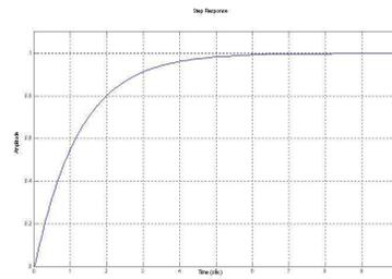
Figure 18. Step response with mixed sensitivity based  $\mathcal{H}_\infty$  controller
