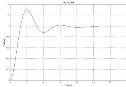
Figure 15. Step response of the identified model using  $\mathcal{H}_\infty$  control
