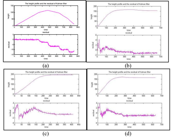
Fig. 6. Kalman filter results under various leakage magnitudes for (a) ON-OFF Controller: for Flow and Heights. (b) P Controller: for Flow and Height. (c) PI Controller: for Flow and Height. (d) PID Controller: for Flow and Height.
