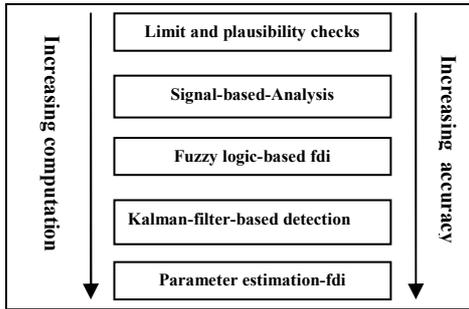
Fig. 2 Execution of diagnostics tasks in the order of increasing computation and accuracy
