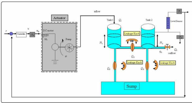
Fig. 1: Two-tank fluid control system
