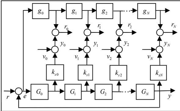
Fig. 3: Sensor Network scheme for the generation of residuals
