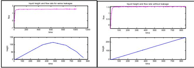
Fig. 4 Input flow rate and the tank height under (a) various degrees of leakage (b) no leakage.
