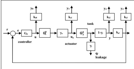
Fig. 5: Sensor Network scheme for the generation of residuals
