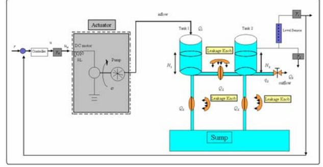
Fig. 3 Process control system: A Lab-scale two-tank system
