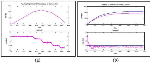
Fig. 4. Kalman filter results for an (a) On-Off and (b) PI Controller: for Flow and Height under various leakage magnitudes
