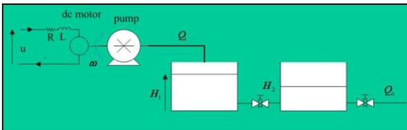
Fig. 1 Two tank fluid system
