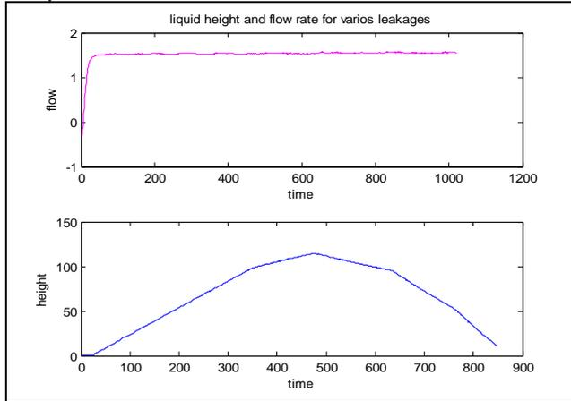
Fig. 4 Input flow rate and the tank height under various degrees of leakage
