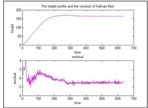
Fig 9:Kalman filter results of PID Controller: for Flow and Height under various leakage magnitudes
