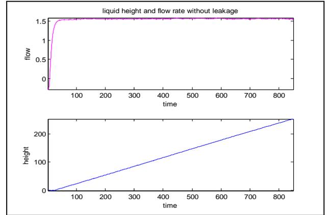
Fig. 5 The flow and the height under no leakage. Note that the height is essentially a ramp
