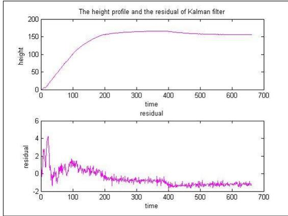
Fig 7:Kalman filter results for P Controller: for Flow and Height under various leakage magnitudes
